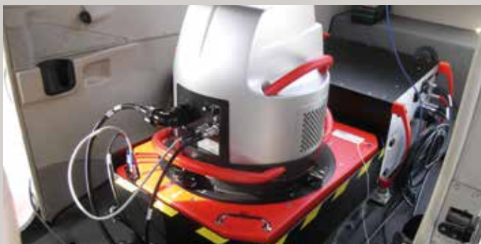
LEICA ADS80 in Cessna 182
